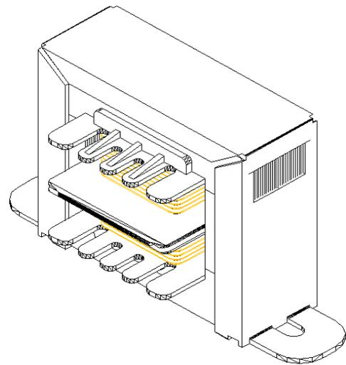
ÁREA ÚTIL DA JANELA:  $2 \times 39,6 \text{ mm}^2$
